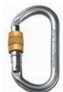
K4241Z005 OVAL STEEL CONNECTOR / screw with screw gate, key lock, zinc plated ⬆ 30 kN ⬆ 9 kN ⬆ 8 kN Gate opening (d): 18 mm 176 g ■ 6,21 oz serial unique number CE 1019 ■ EN 362
