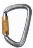
K4081ZD D STEEL CONNECTOR / triplelock with triple lock gate, key lock, zinc plated ⬆ 50 kN ⬆ 13 kN ⬆ 20 kN Gate opening (d): 25 mm Weight: 267 g ■ 9.42 oz serial unique number CE 1019 ■ EN 362
