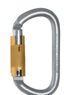
K4241Z007 OVAL STEEL CONNECTOR / triplelock Triple lock gate, key lock, zinc plated Gate opening (d): 18 mm Weight: 176 g ■ 6.21 oz ⬆ 30 kN ⬆ 9 kN ⬆ 8 kN serial unique number CE 1019 ■ EN 362
