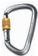
K4080ZD D STEEL CONNECTOR / screw with screw gate, key lock, zinc plated ⬆ 50 kN ⬆ 13 kN ⬆ 20 kN Gate opening (d): 25 mm Weight: 255 g ■ 9 oz serial unique number CE 1019 ■ EN 362
